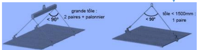
Fig.25 - Concept 5 : Flux de manutention
